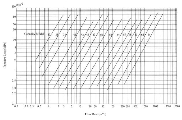
Note) This diagram indicates the case of water at Specific Gravity: 1.00, Viscosity: 1.00mm²/s.
