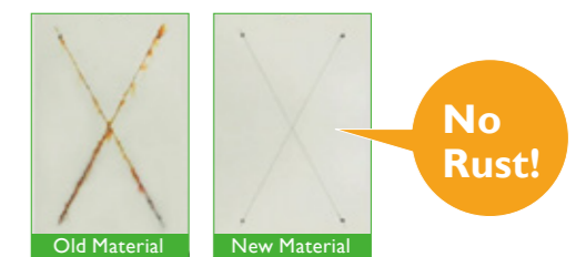
Results of Salt Spray Long-life Test Based on Japanese Standard
